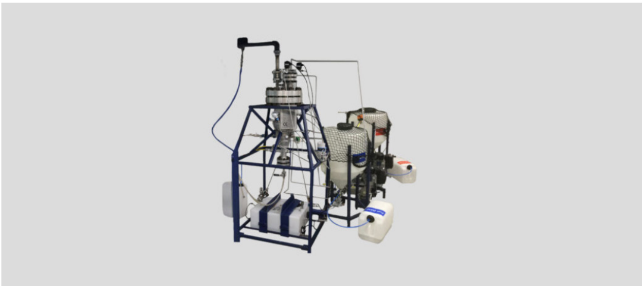
System setup H2Fuel reactor
